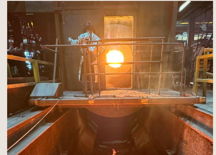
Technician in protective clothing controls the process where the purified slag is heated to 1,600 degrees. Photo: Swerim
